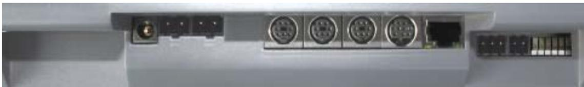
ECoSlot-expansion port for mobile station receiver module
